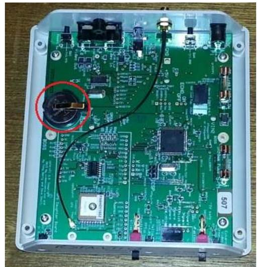
Simply pull on the tag to activate the backup battery.
