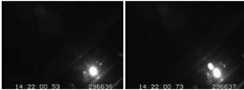
If you see the LED illuminate within one field of UTC change, then your camera sends video as it happens. If the LED illuminates two fields or more after UTC change, then the camera is an accumulating camera. YOU NEED TO KNOW how many fields the camera accumulates before sending the image.
